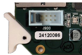
Figure 4-2 Boot-Loader jumper location
