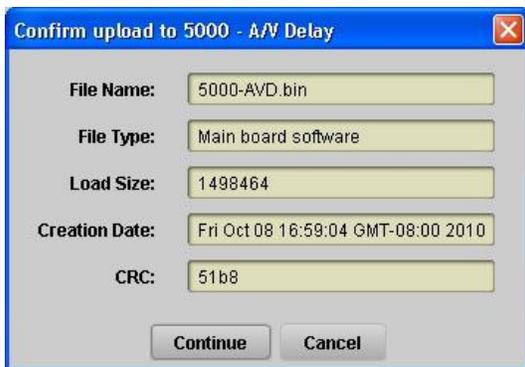
5. Click **Continue** to begin installing the new firmware. When the installation is complete the 5000-Series card will automatically reboot with the new firmware. Verify that the new version numbers are displayed on the Dashboard™ control *Product* menu.
